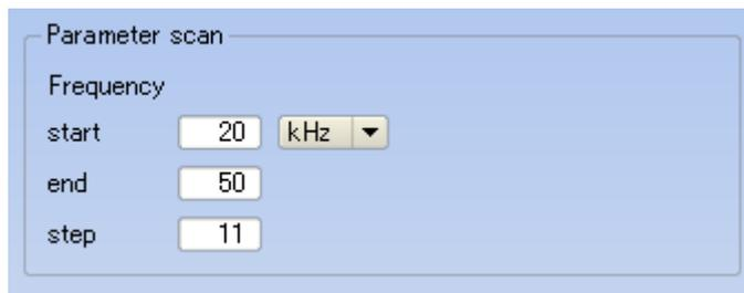
For example, if you input values as above, the cantilever is oscillated with divided the range from 20.0 kHz to 50.0 kHz into eleven points. Thus you can set a sequence of frequencies.
